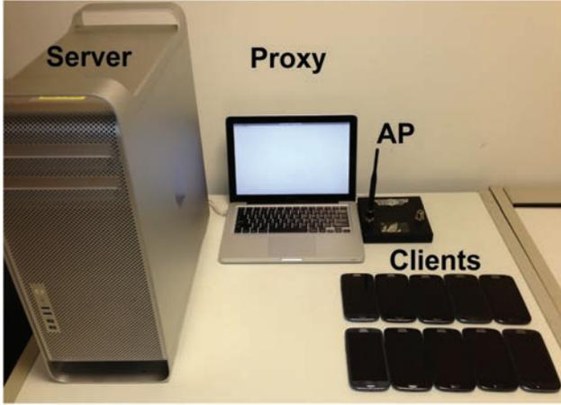
Fig. 8. System setup.
